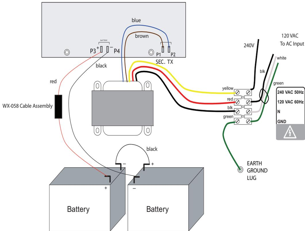
**Figure 54 Power Supply Connections**
