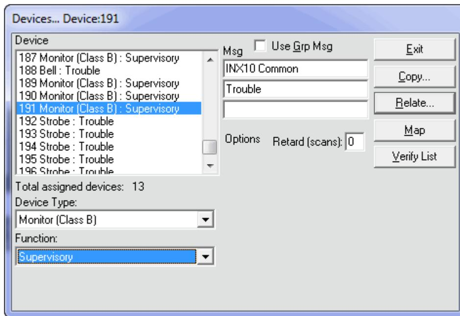
Figure 37 Secutron MR-2100/2200/2900 Configurator Settings - INX-10A Two Stage with Enhanced Reporting and Power Supply Addressing
