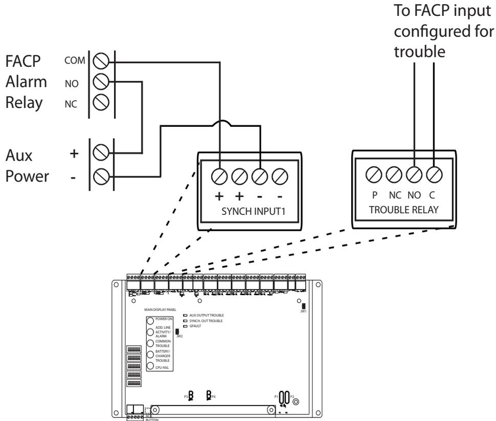
Figure 48 Relay Contact Activation from FACP - Single Stage
