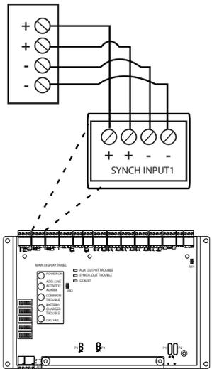
Figure 44 Synchronized Input from FACP Wiring - Class A
