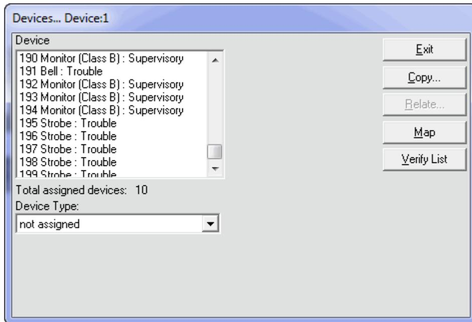
**Figure 19 Secutron MR-2100/2200/2900 Configuration Settings - INX-10A Single Stage with Enhanced Reporting**
