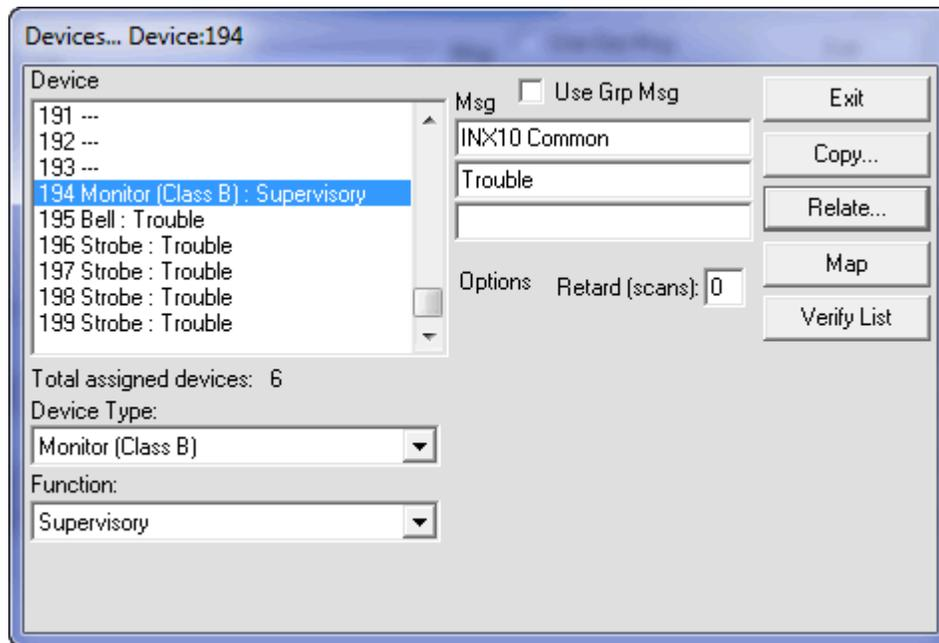
**Figure 22 Secutron MR-2100/2200/2900 Configurator Settings - INX-10A Single Stage with Basic Reporting and Power Supply Output**
