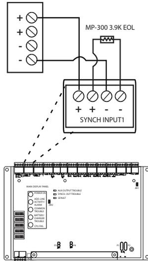
Figure 43 Synchronized Input from FACP Wiring - Class B
