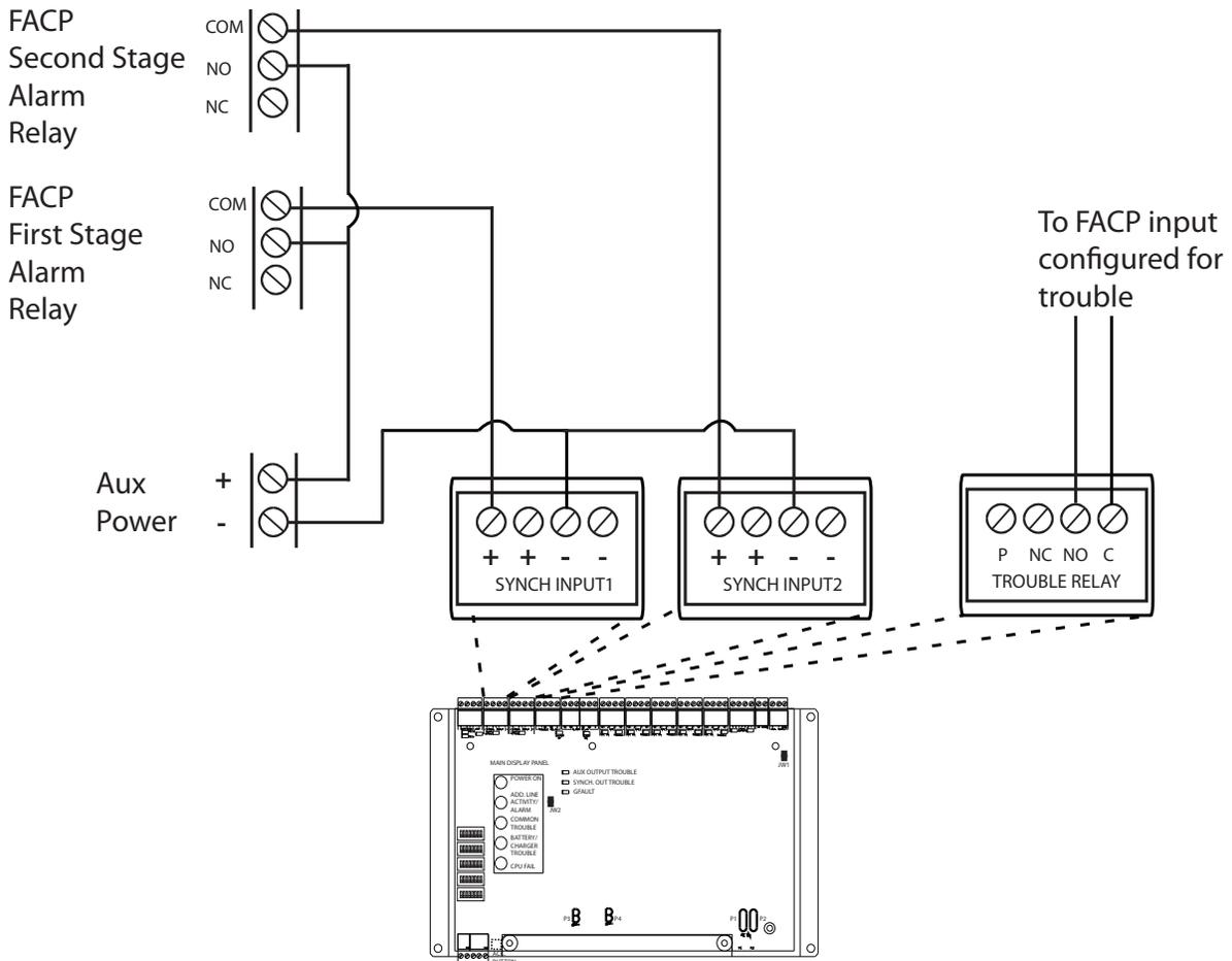
Figure 49 Relay Contact Activation from FACP - Two Stage
