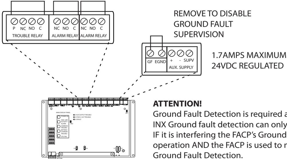
Figure 50 Relay, Ground Supervision and Auxiliary Supply Wiring
