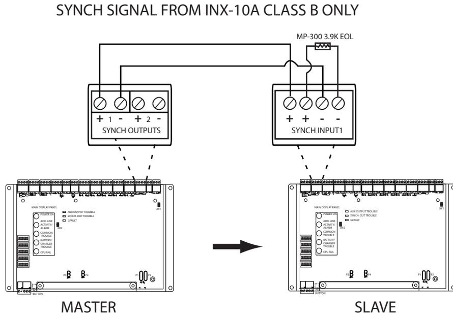
Figure 45 Synchronized Input from INX-10A Wiring - Class B Single Slave
