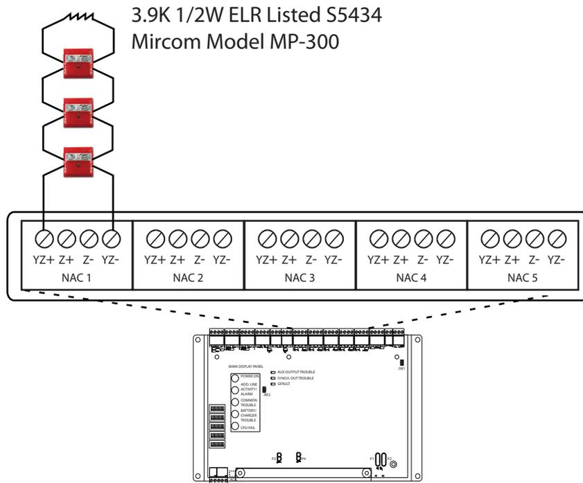
Figure 52 NAC Circuit Wiring - Class B
