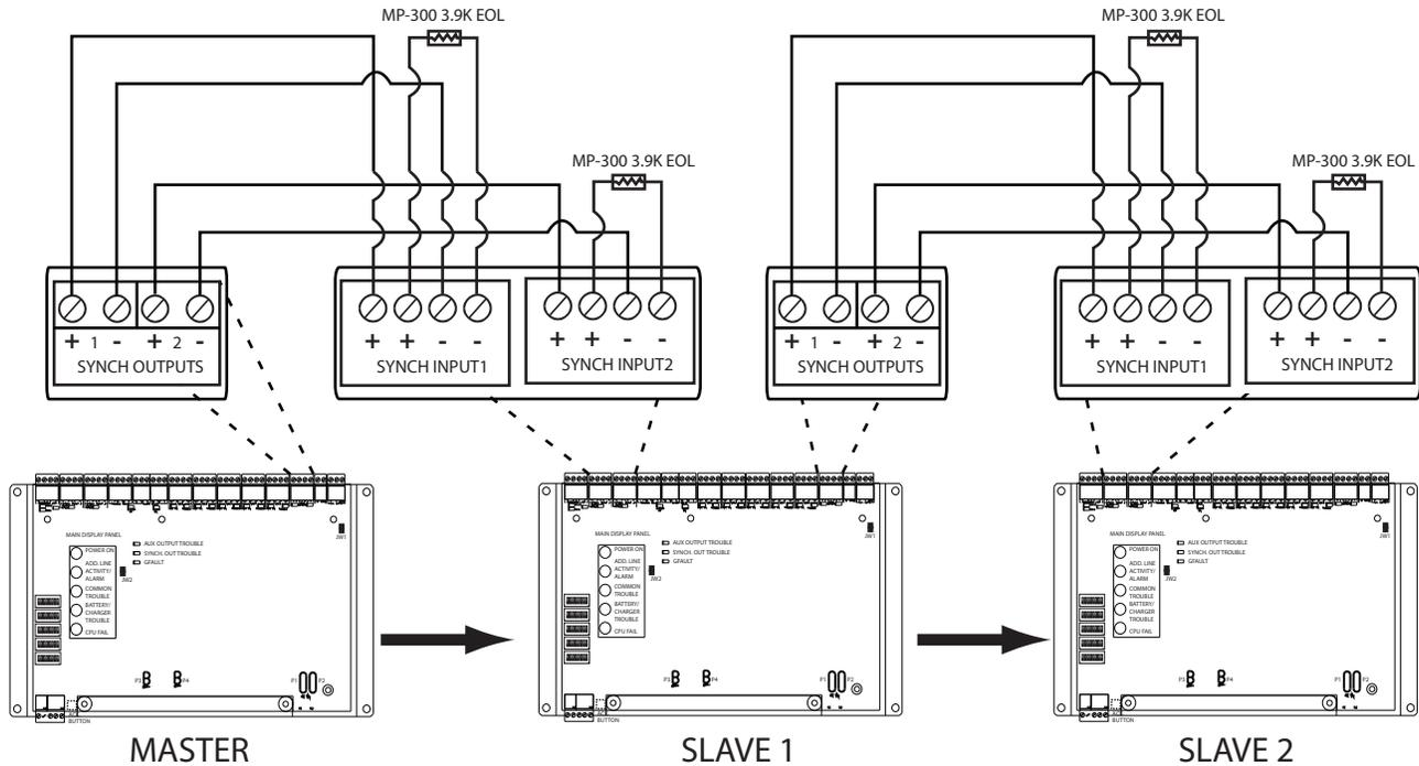
Figure 47 Synchronized Input from INX-10A Wiring - Class B Multiple Slaves
