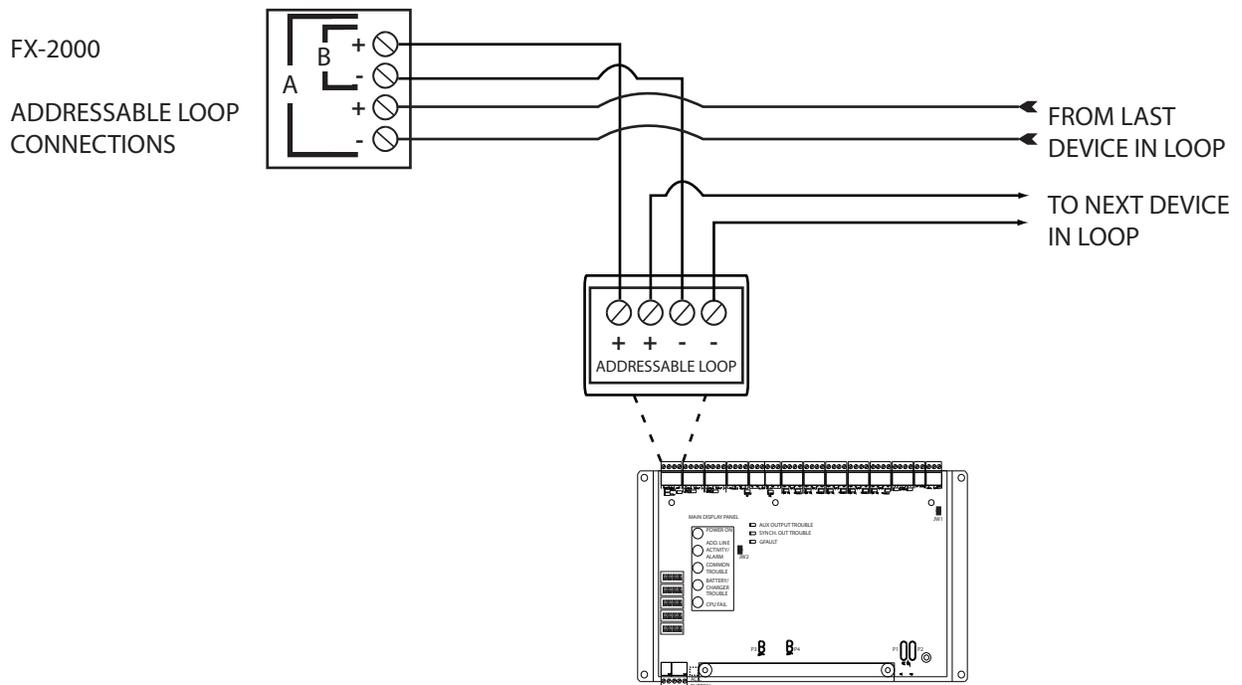
Figure 42 SLC Loop Wiring - Class A
