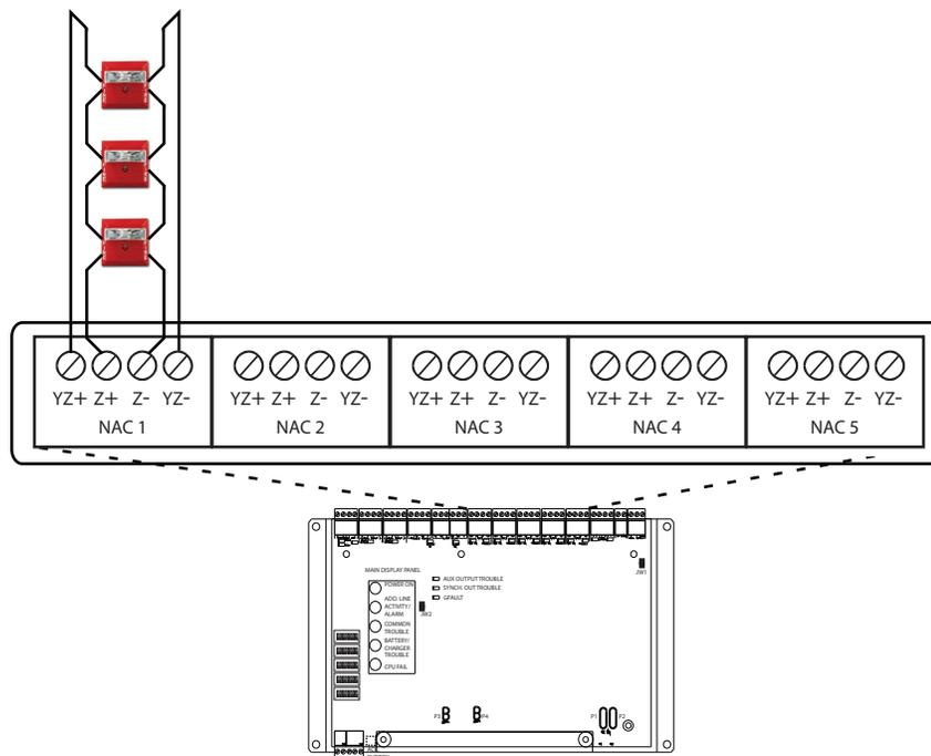
Figure 53 NAC Circuit Wiring - Class A
