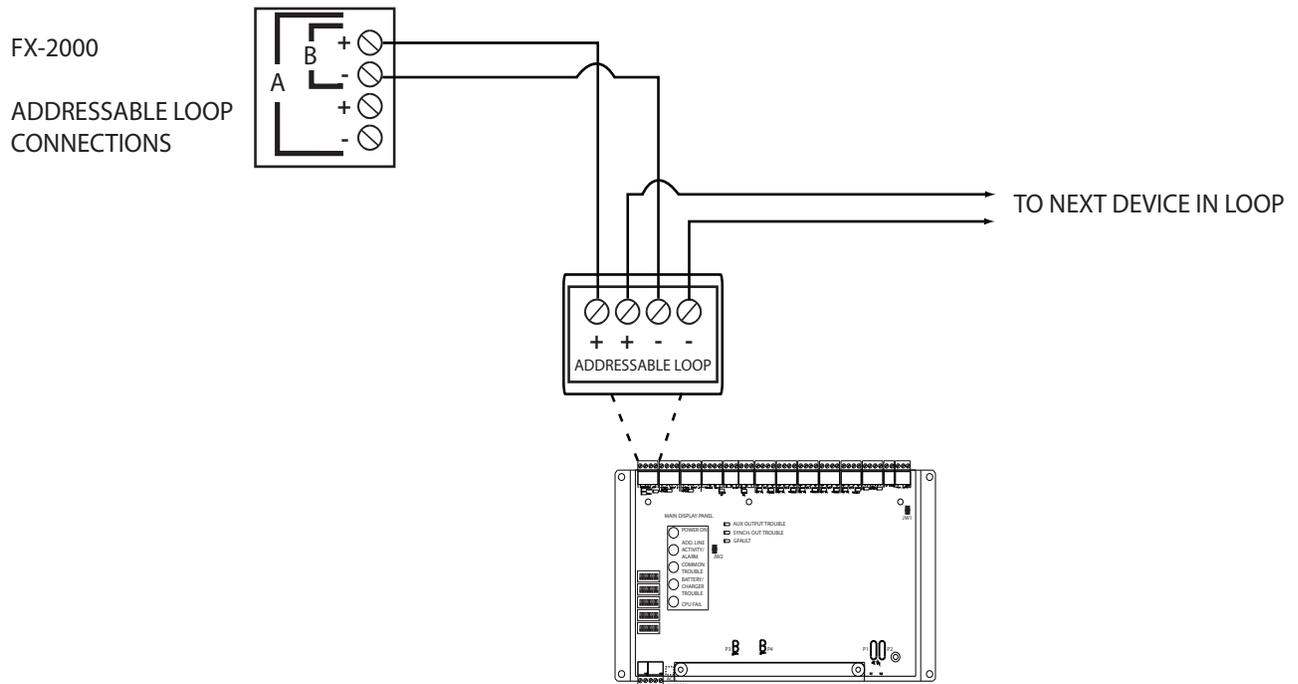
Figure 41 SLC Loop Wiring - Class B
