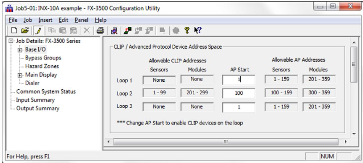
**Figure 14 Configurator CLIP/Advance Protocol Device Address Space window**
