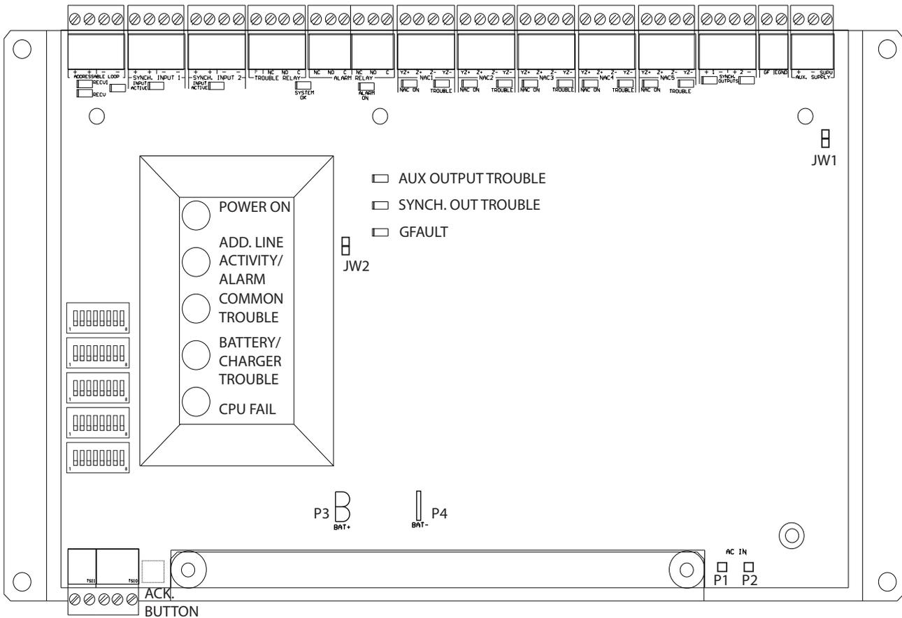
Figure 6 INX-10A Chassis Board Connectors and Jumpers
