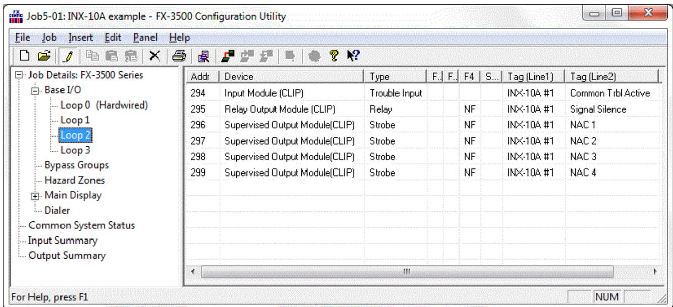
**Figure 23 FX-3500/3500RCU/MR-3500/3500RCU Configurator Settings - INX-10A Single Stage with Basic Reporting and Power Supply Output**
