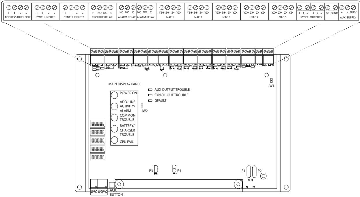
Figure 40 Main Board Terminal Blocks
