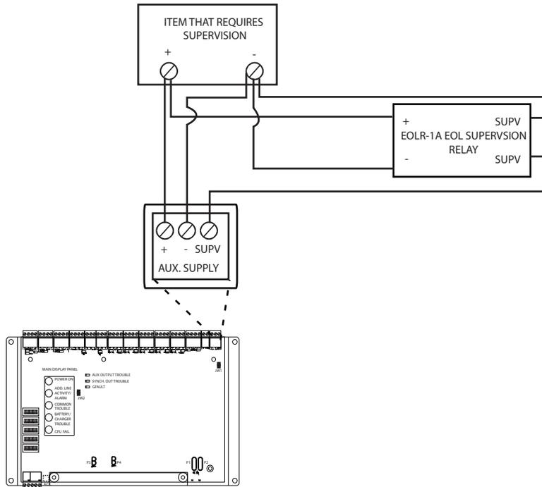
Figure 51 Relay, Ground Supervision and Auxiliary Supply Wiring
